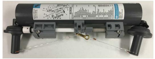
Non-metallic free-flushing sampling bottles activated by GO Devil Messenger (1000-MG) when individually or serially attached to hydrocable. Sequential closure by remote command with model 1015 or 1018 Rosette multibottle array.
