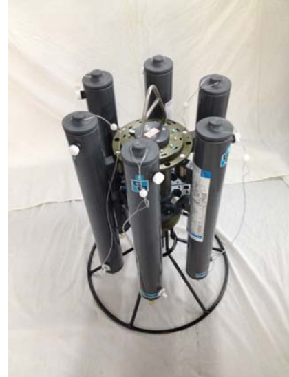
Lightweight rosette with Niskin bottles
