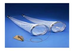
It has single window, slightly offset, so you can easily pour out the content. The window are covered by a net, according to the mesh size of the plankton net. The windows are protected by stainless steel net at the outer side.
